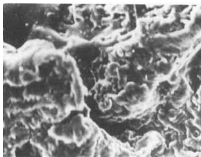
FIGURE 7 SEM Photograph of the blend Sample No. 1 ( \times 1000 ).
